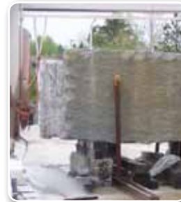
Large blocks are cut into slabs with saws similar to this.
